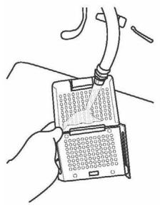
10. Remove the pluggable heater from the instrument and use a 1-5% (v:v in water) household bleach solution spray bottle to spray the pluggable heater with bleach.
